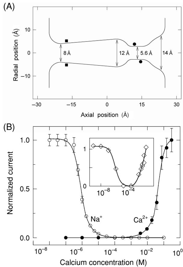
**Fig. 7.8** Brownian dynamics model of an L-type calcium channel. (A) The channel shape contains a narrow portion of the pore surrounded by the charge from the four glutamate residues (circles). (B) Results from Brownian dynamics simulations in mixed  $\text{Na}^+$  and  $\text{Ca}^{2+}$  solution reproduce the “anomalous mole fraction” behavior seen in the experimental data (Almers et al., 1984). Figures from Corry et al. (2001).
